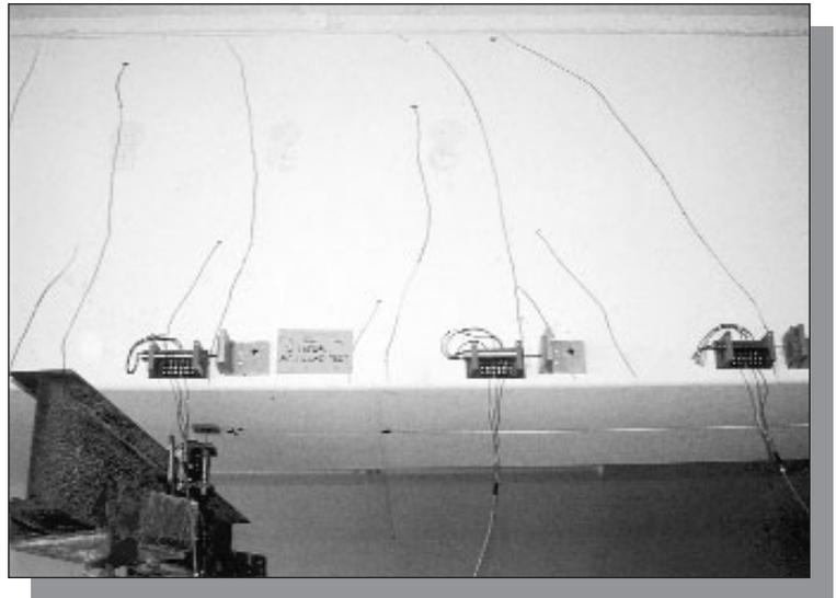
Figure 2 - Mid-span of post-tensioned beam with cracking outlined. LVDT's are in place to monitor crack widths during load test.
