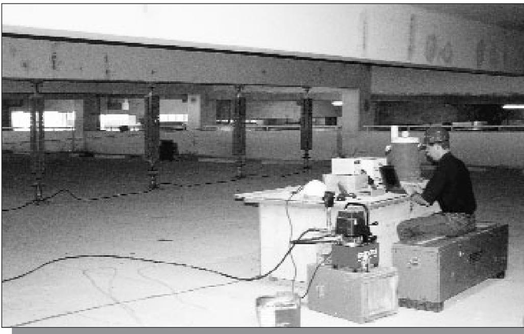
Figure 3 - Load test consisting of hydraulic jacks coupled together with manifolds to apply an equivalent uniform load across the beam.
