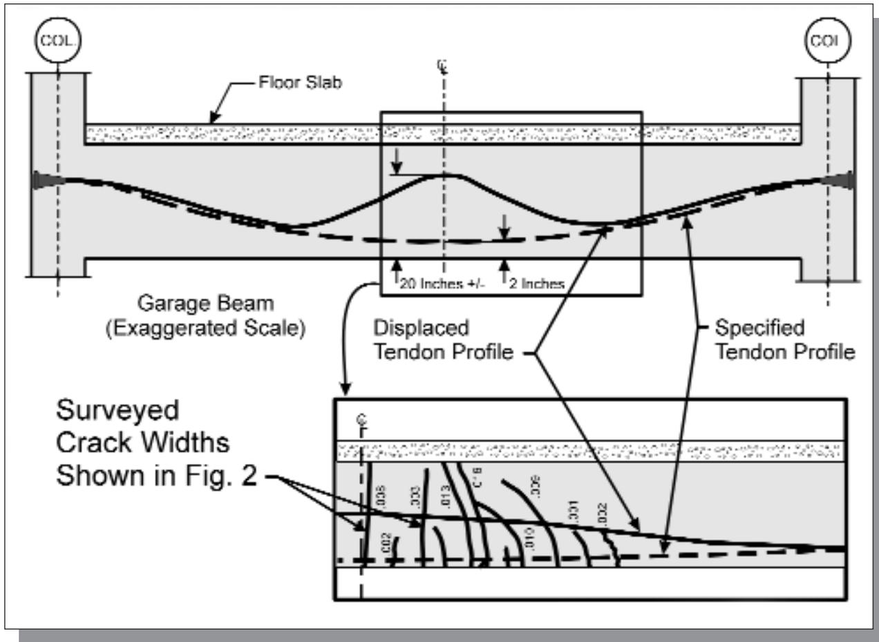
Figure 4 - Typical beam elevation showing displaced tendon profile and surveyed crack widths.
