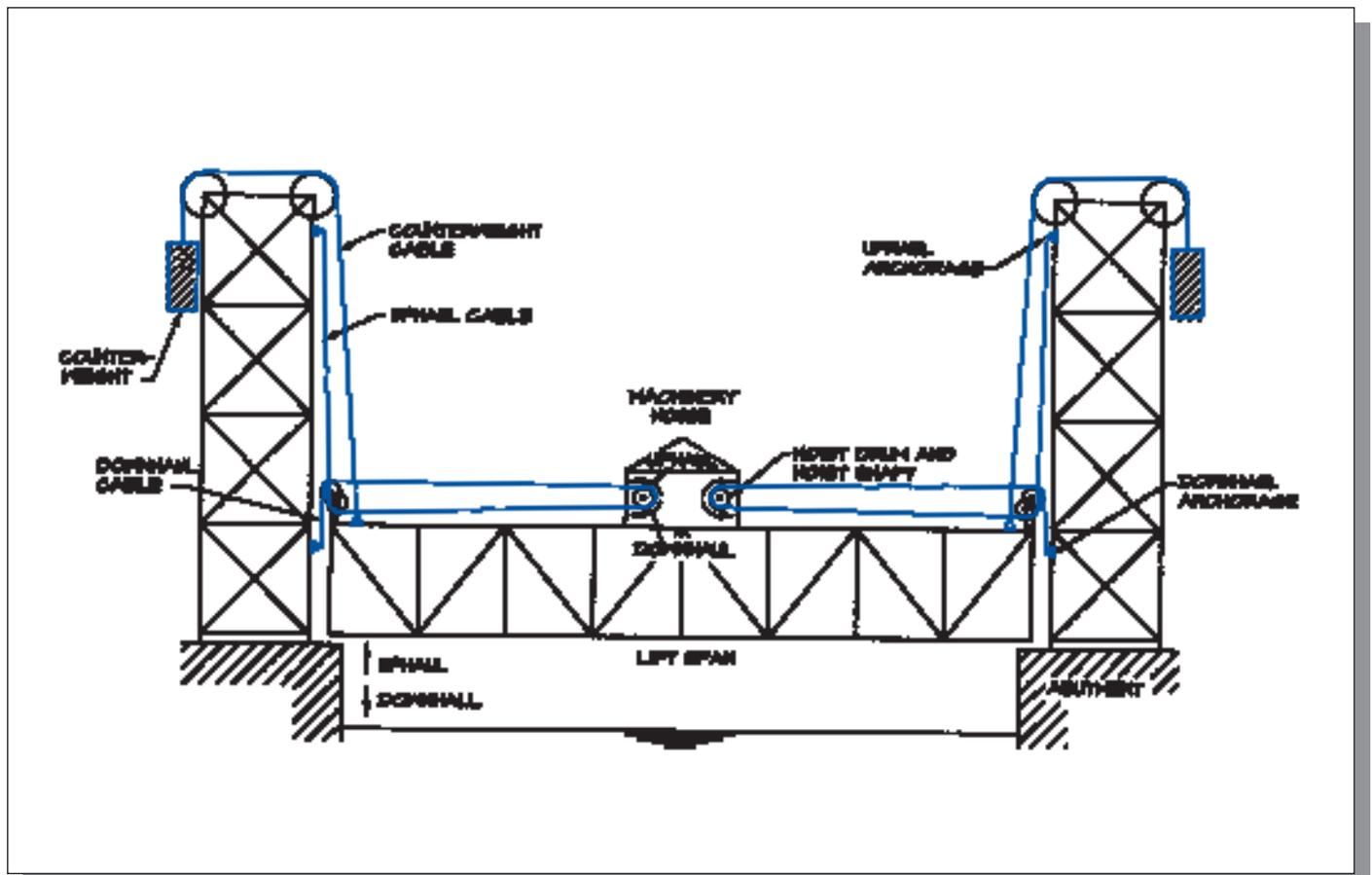
Figure A - Schematic View of a Typical Lift Bridge.
