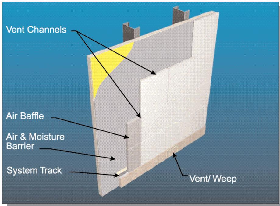
Figure 4 – Example of pressure equalized rain screens
