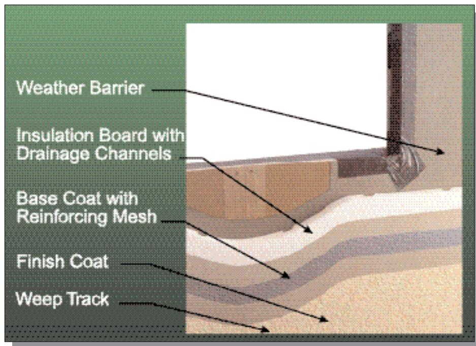
Figure 3 – Example of water managed or drainage systems.
