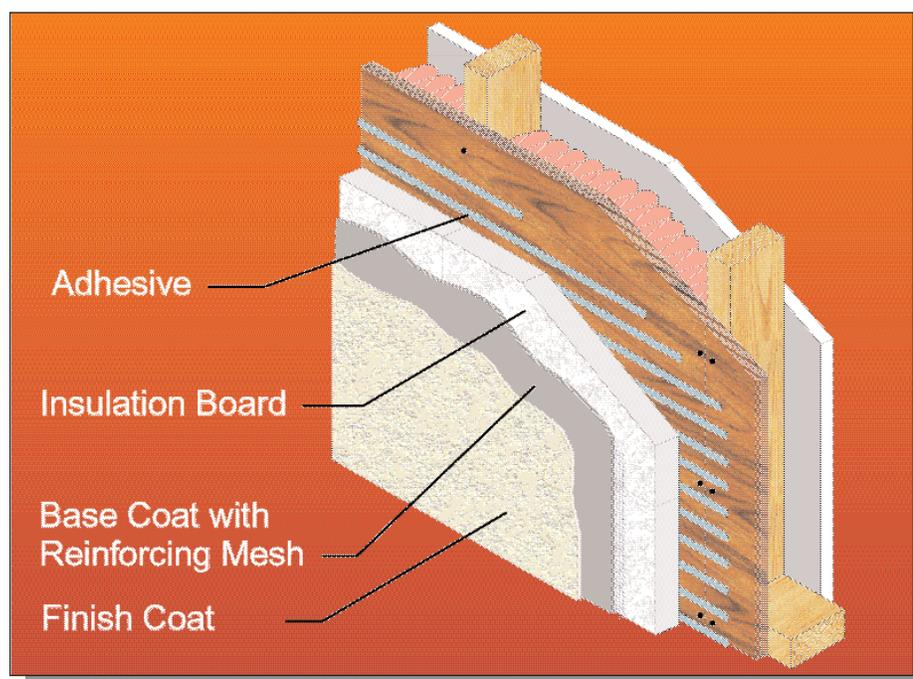
Figure 2 – Example of barrier system.
