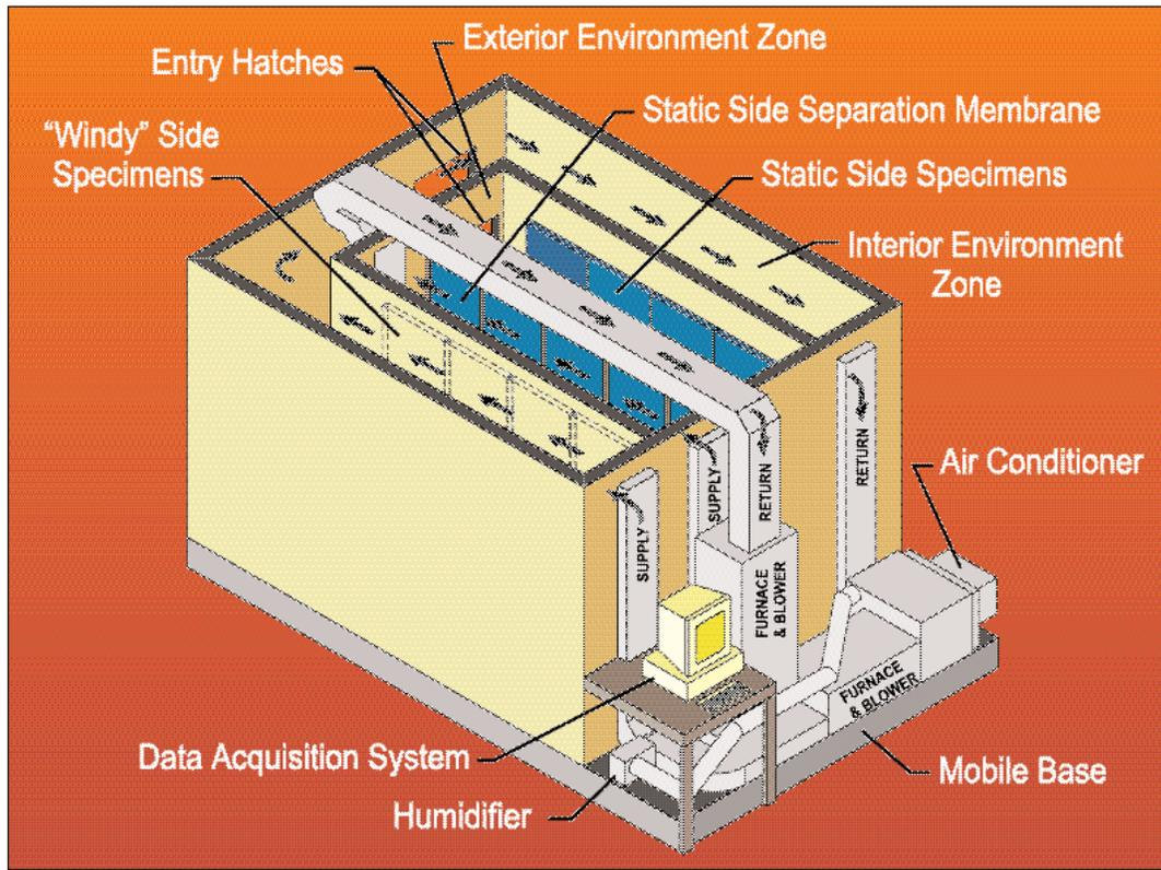
Figure 5 – RRJ's climatic test chamber used to compare dry-out potentials for various cladding materials.
