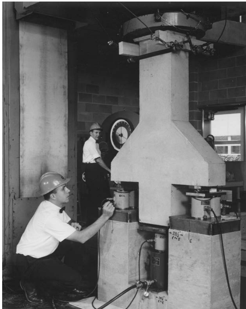
Chuck Rath performing early concrete corbel research.
