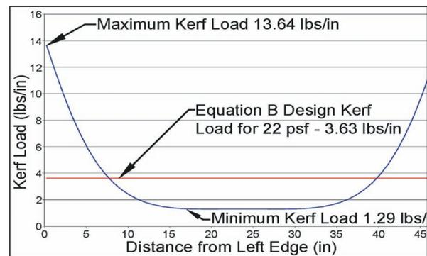
Figure 3—Actual kerf loads compared to calculated loads based on simplified assumptions.
