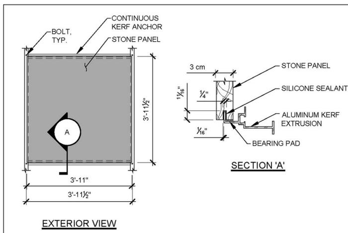
Figure 1— Example of a full-width kerf anchor configuration.
