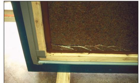
Figure 2—Progressive cracking of a full-width kerf anchor configuration during laboratory testing.
