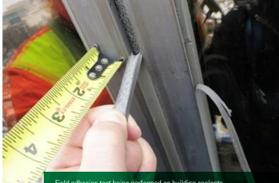
Field adhesion test being performed on building sealants
