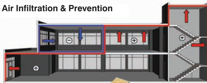
Figure 4, above: Differential pressures within a building.
